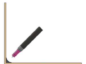
▲ Flat Corner Welding
